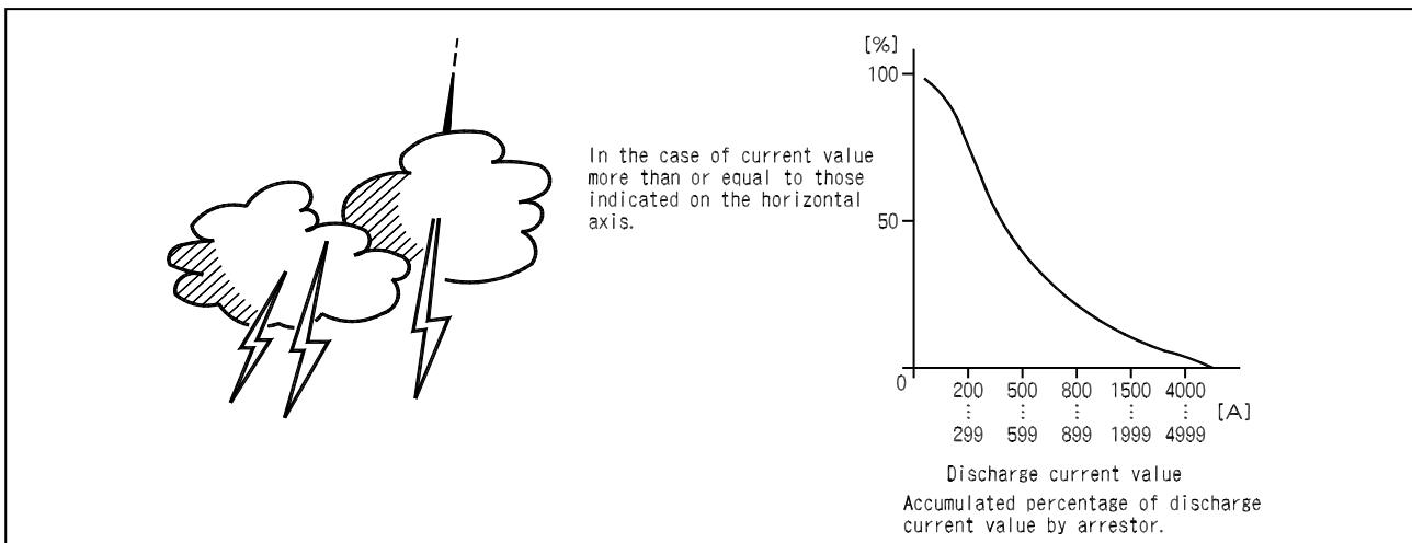
The statistical result of thunder accident which happened to low voltage circuit in national main power stations according to a report on thunder accident of low voltage controlling circuit] released by Investigation Committee for thunder accident, IEEJ;
