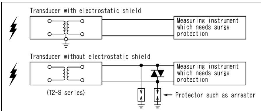
If there is the possibility for an induced lightning surge occurring on input of an AC transducer, take measures as the figure in the left shows.
