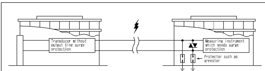
An AC transducer, a sensor transducer or a signal transducer with output line surge protection does not need a protector at transducer output side. Constant current output type which is normal mode noise resistant, such type is the choice in the case of transmitting an output to a distant place.
