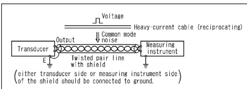
Please ground either one of transducer side and instrument side of the shield.
