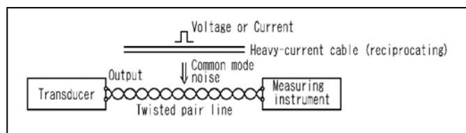
► Effect of using twisted pair line with shield
