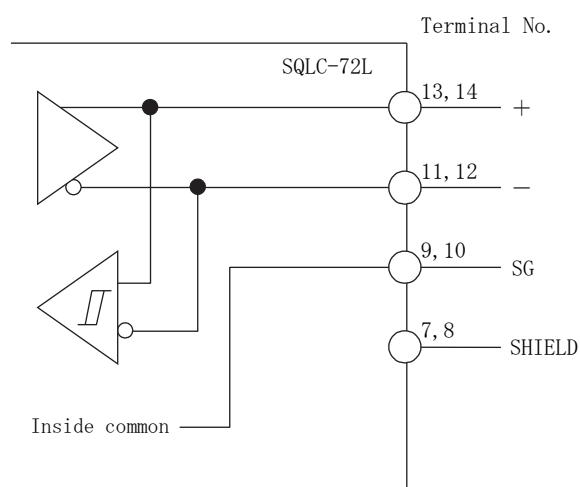
Communication output terminals 7 and 8, 9 and 10, 11 and 12, 13 and 14 are connected internally. When transition wiring, connect as shown below. Connect the attached resistor to the terminal equipment as shown in the figure.
