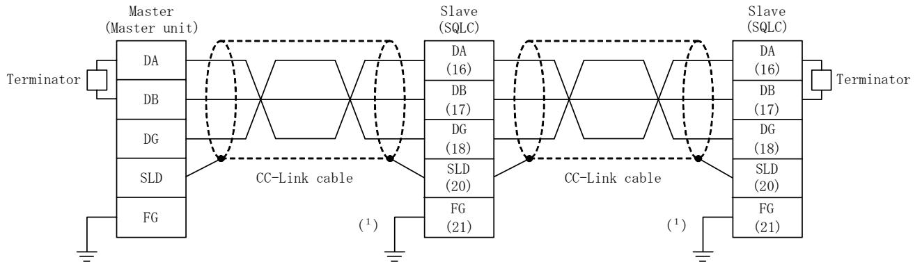
Note<sup>(1)</sup> FG is equivalent to the function ground, so we recommend a dedicated ground or shared ground.
