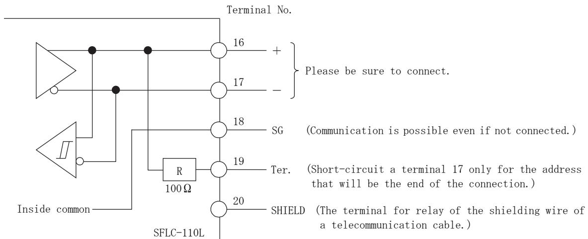
(Termination resistor is connected by short-circuiting terminals 17 and 19.)
