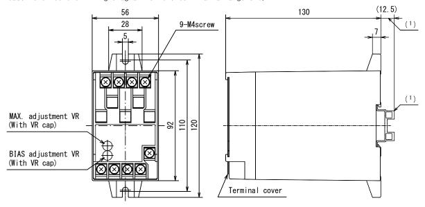
Note(1) Dimensions when IEC/DIN rail (height 15mm) is installed. (Please use a rail with a width of 35mm) The terminal cover is standard equipment.
