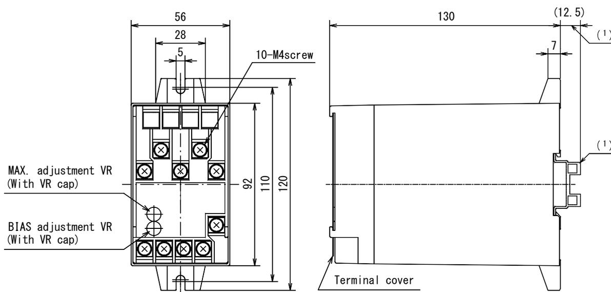
Note<sup>(1)</sup> Dimensions when IEC/DIN rail (height 15mm) is installed. (Please use a rail with a width of 35mm)
