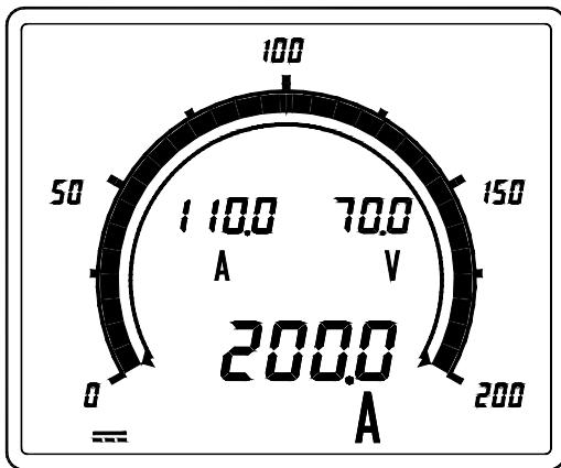
In case of display scaling setting 0 - 200.0A of input 1.
