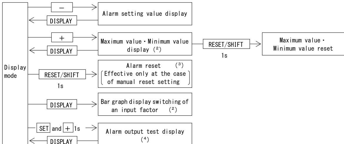
Note (2) By "DISPLAY switch function change setting", in case it is set as "+ : bar graph display change" and "DISPLAY : maximum and the minimum value", if DISPLAY is pushed, maximum and the minimum value will be displayed.
