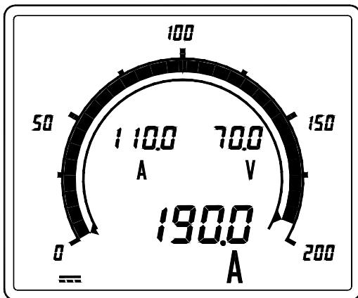
The scale of 200 is selected because there is no scale 190. (The nearest bar scale including 190.0 values is selected.)
