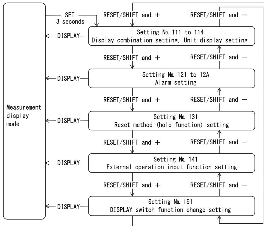
Setting mode 1 is selected by pushing [SET] switch for longer than 3 seconds. For shifting the setting items, push [+ ] and [RESET/SHIFT] or [- ] and [RESET/SHIFT] together. The present mode can be returned to the display mode by pushing [DISPLAY] switch.
