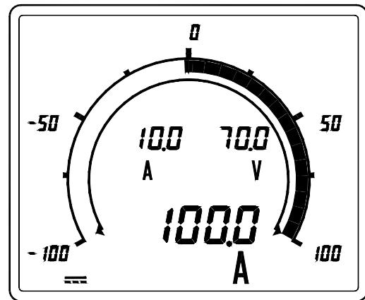
In case of display scaling setting -100 to 0 to 100.0A of input 1.
