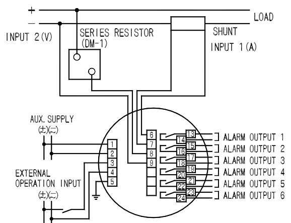
From the measurement value of the DC current input 1 (A) and the DC voltage input 2 (V), a DC power is calculated, and display.
