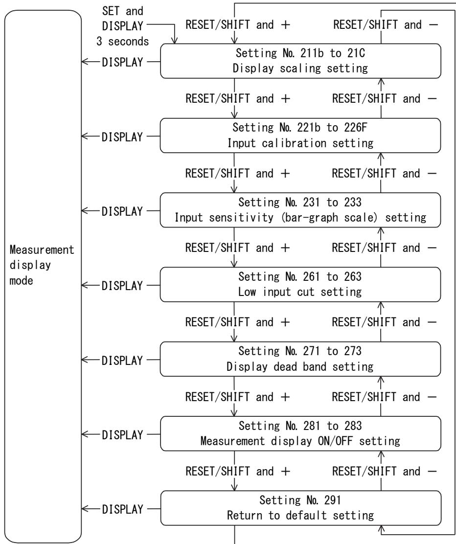
If [SET] switch and [DISPLAY] switch are simultaneously pushed for more than 3 seconds continuous, it will become the setting mode 2 from display mode.
