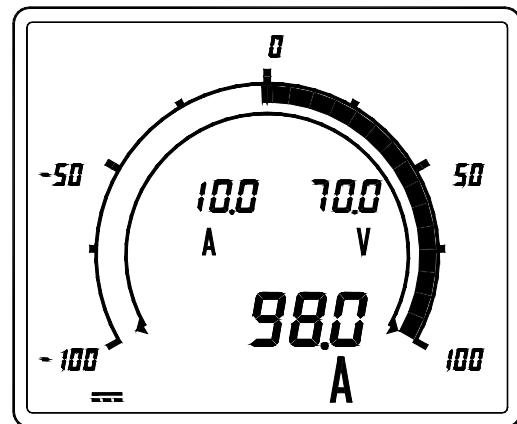
The scale of 100 is selected because there is no scale 98. (The nearest bar scale including 98.0 values is selected.)
