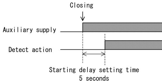
(2) Starting delay time 5 seconds < Contact delay time 10 seconds
