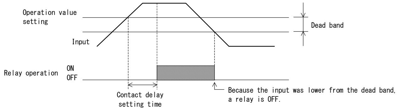
(2) Relay operation in manual reset setting. (Output mode : Excitation, H)
