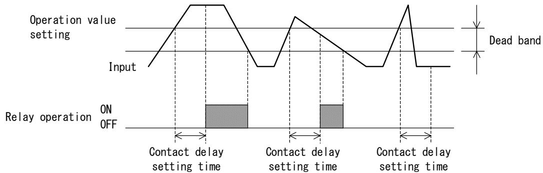
(2) Relay operation in shortage-input detection. (Output mode : Excitation, L)
