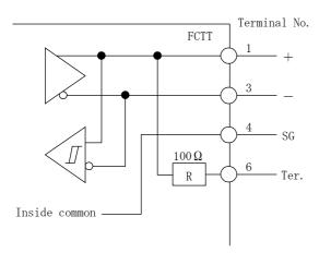
The termination resistor (100  $\Omega$ ) is connected by short-circuiting a terminal 3(-) and a terminal 6(Ter.).
